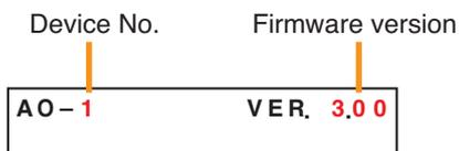
Displays the SX-2000AO's current operation status, output level, etc. (See the separate Operating Instructions, "SX-2000AO Audio Output Unit.")
