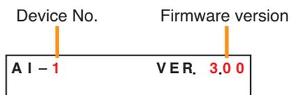
Displays the SX-2100AI's current operation status, input level, etc. (See the separate Operating Instructions, "SX-2100AI Audio Input Unit.")
