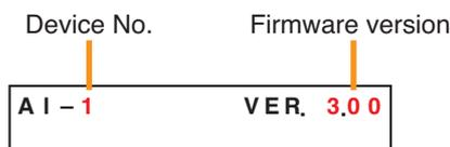
Displays the SX-2000AI's current operation status, input level, etc. (See the separate Operating Instructions, "SX-2000AI Audio Input Unit.")
